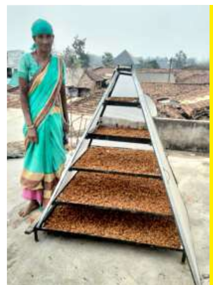
Field trials of Pyramid Solar Dryer
